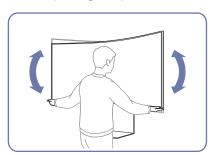
• Hold the bezel at both side edges and adjust the monitor angle until the screen becomes level. (Be careful not to directly hold the LCD display.)
