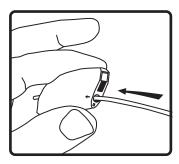
5. Thread hanging or safety cable through SpeedClamp™ mechanisms as shown.
