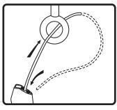
**6.** Attach the hanging cable by securing it and safety cable to structure as shown.
