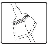
2. Slip terminal weather boot over signal wire. For environmental applications, put RTV silicone around nipple and base when installation is complete.
