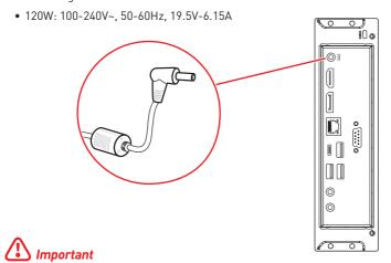
When unplugging the AC power cord, always hold the connector part of the cord. Never pull the cord directly.
