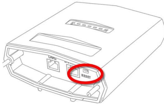
Figure 8. Cisco FM3200 Base (Hardware RESET button port)
