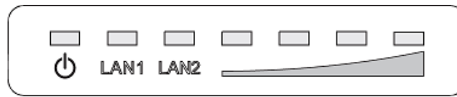
Figure 6. Status and link/boot LEDs
