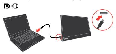
2) Connect the USB-C port of mobile phone and M14d with a USB type-C cable. (Electronically marked cable, current rating: 5A)
