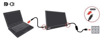
2) Connect Type-C power adapter to the left or right side of M14d and connect M14d to the mobile phone with a USB-C cable. (Electronically marked cable, current rating: 5A)
