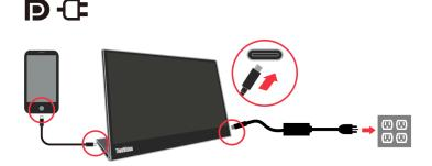
**NOTE:** When you encounter abnormal charging condition, please check your power capacity of power adapter connected with M14d and make sure it is enough for M14d and other devices.
