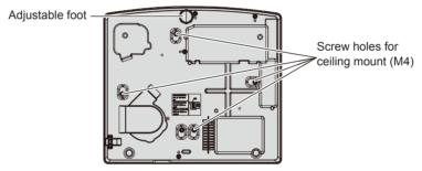
Positions of screw holes for ceiling mount and adjustable foot
