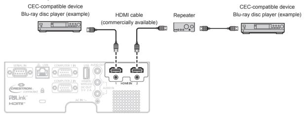
Connection example with CEC-compatible device
