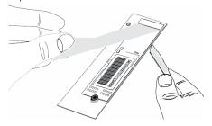
4. Secure the tray in place with the included screws. Optionally, paste the faceplate over the LEDs with the acrylic tape side of the plate.
