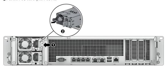
3 Prepare a new PSU. Insert it into the empty slot until you hear a click.
