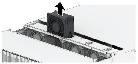
**5** Prepare a new fan and slide it into FS3410. Make sure that the fan is aligned properly.
