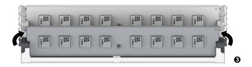
**Note:** Hold the memory module by its edges and avoid touching the gold connectors.
