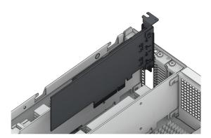
**Note:** Confirm that the connector is fully inserted. Otherwise, the network interface card might not be able to function properly.
