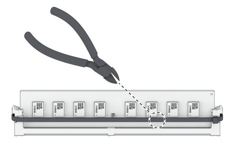
Note: Avoid touching any components on the motherboard when cutting the cable tie.
