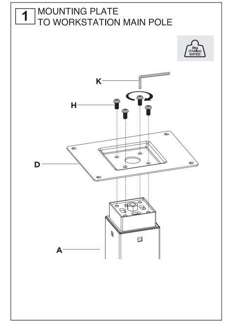
MOUNTING POLE+PLATE TO UNDERSIDE OF TABLE
