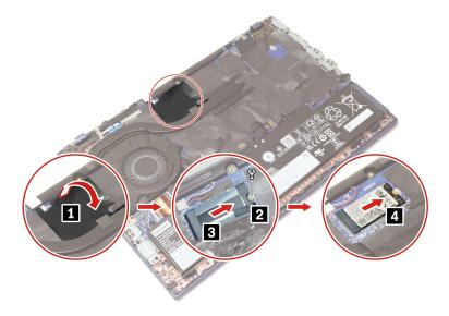
Before installing: If you replace the M.2 solid-state drive, ensure the thermal pad upper and down the solidstate drive are attached in place.
