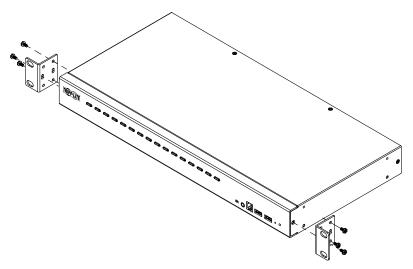
Place the KVM switch in the rack. Position it so that the holes in the mounting brackets line up with the holes in the rack. Secure the mounting brackets to the front of the rack.
