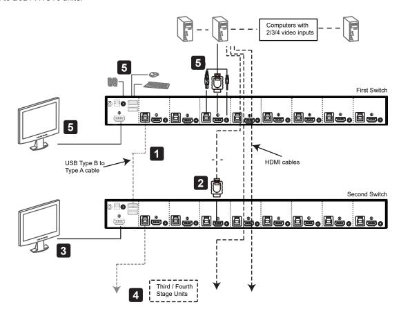
1 Use a standard USB Type-A to USB Type-B cable to connect the Port 8 USB Type-B port on the First-Stage unit to the USB Type-A port in the Console Ports Section of the second switch.
