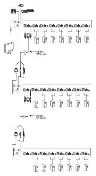
Once you have finished cabling up (see section **7.3.2 Two-Stage Cascade Installation**), power up according to the following sequence:
