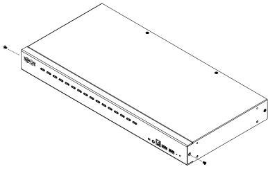
2 Use the M3 x 6 Phillips hex head screws supplied with the rack mounting kit to attach the rack mounting brackets onto the sides near the front of the unit.
