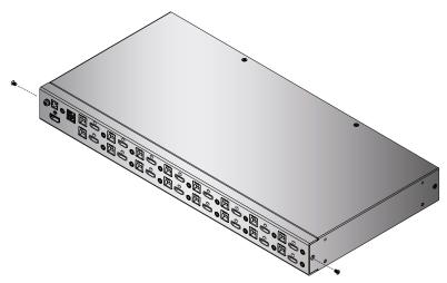
2 Use the M3 x 6 Phillips hex head screws supplied with the rack mounting kit to attach the rack mounting brackets onto the sides near the rear of the unit.
