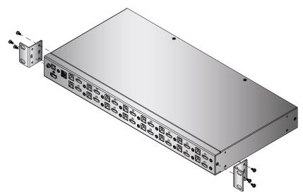
Place the KVM switch in the rack. Position it so that the holes in the mounting brackets line up with the holes in the rack. Secure the mounting brackets to the rear of the rack.
