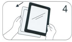
Once the iPad is inside the rear cover, place the internal front cover on top and gently clip all four sides into position.
