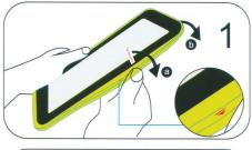
Remove the external silicone sleeve by peeling it away from the internal hard case
