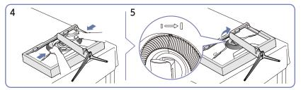
Attach the decoration cover in the direction of the arrow and turn it in clockwise according to the mark.
