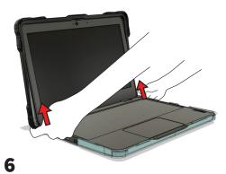
Push the left and right side clips down past the device, one side at a time, to release it from
