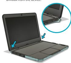
**3**Start sliding the top case off by pushing up with your fingers on the bottom corners.
