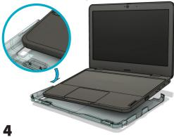
Close the device screen and carefully press the rear corner clips to snap onto the keyboard.
