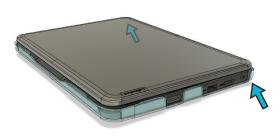
Close the case and press on the clips located on the bottom of the top case. Make sure the clips are securely attached
