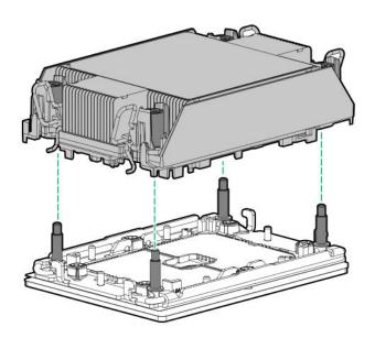
**d.** Using a T-30 Torx screwdriver, tighten the nuts.
