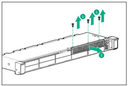
Install the 8SFF display port/USB/optical blank option.
