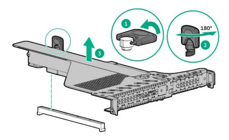
**8.** Remove the PCIe blank from slot 1 on the primary riser cage.
