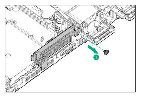
Install the full height PCIe x16 riser cage latch.
