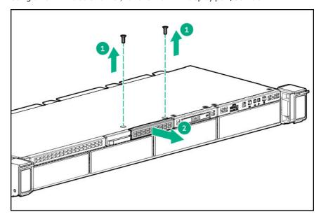
Install the 4LFF display port/USB module.
