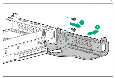
If installed, remove the low-profile riser cage.
