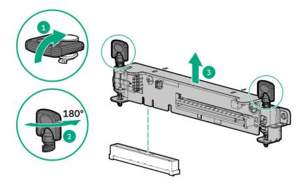
Lift and remove the secondary riser cage latch.
