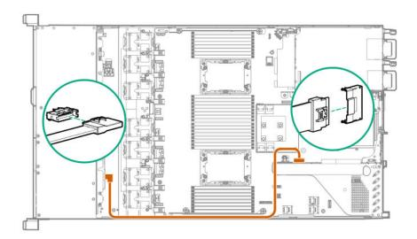
8SFF x1 Tri-Mode U.3 backplane to type-p controller on slot 2
