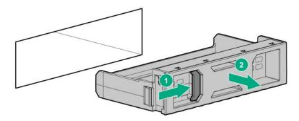
Figure 2: Removing an LFF drive blank
