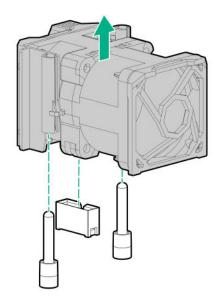
Remove fan blanks from the fan bays, if installed.
