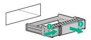
Figure 1: Removing an SFF drive blank
