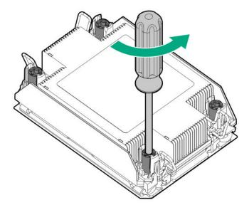
**c.** Remove the processor heatsink assembly.
