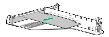
**7.** Remove the existing riser board from the riser cage.
