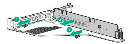
Install the optional riser board in the riser cage.
