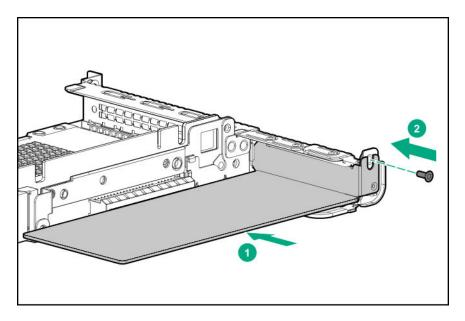
**10.** Install the PCle riser cage into the server.
