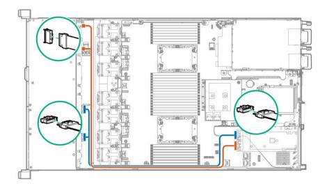
4LFF to a type-p slot 2 controller cabling example
