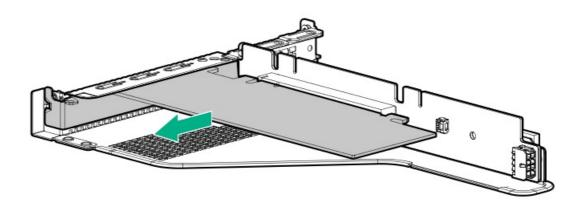
8. Remove the existing riser board from the PCI riser cage.
