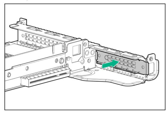
9. Use a T-10 Torx screwdriver to Install the expansion board.
