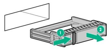
Figure 2: Removing an LFF drive blank
