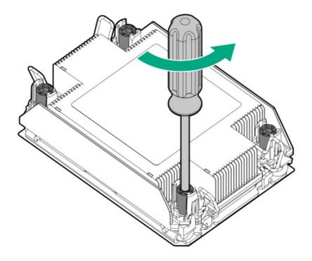
c. Remove the processor heatsink assembly.
