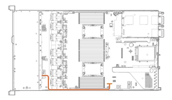
LFF front display port/USB cabling
