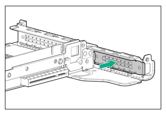
9. Install the DSC-25 card into the PCIe slot.
