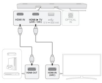
3 Press the Function D button repeatedly until "HDMI" appears on the status display.
