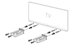
Place the product on the brackets. Position the product on the brackets so the screw holes on the bottom of the product align with the screw holes on the wall bracket.
