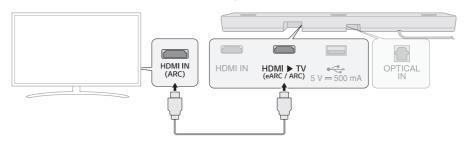
2 Press the Function D button repeatedly until "OPT/HDMI ARC" appears on the status display.
