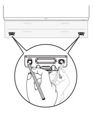
**4** Drill screw holes in the marked positions on the installation guide.
