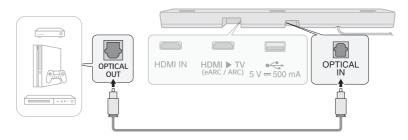
2 Press the Function D button repeatedly until "OPT/HDMI ARC" appears on the status display.
