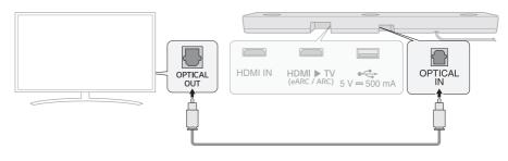
3 Press the Function Dutton repeatedly until "OPT/HDMI ARC" appears on the status display.
