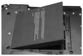
2. Press the battery down until it snaps into place.
