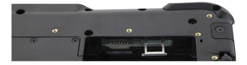
6. Install the battery in the tablet. See Replacing the Battery on page 29.
