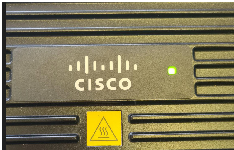
Figure 5: Top Cover LED
