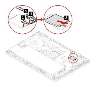
Note: After installation, ensure that you connect the orange cable to the connector labeled Orange on the card, the blue cable to the connector labeled Blue, the white and grey cable to the M1 connector, and the black and grey cable to the M2 connector.
