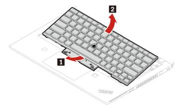
7. Put the keyboard on the palm rest as shown and detach the connectors. Then, remove the keyboard.
