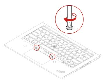
5. Take the new TrackPoint buttons out of the new keyboard packaging. Install the TrackPoint buttons as shown.
