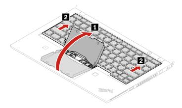
6. Pivot the keyboard slightly upward as shown by arrow **II.** Then, turn over the keyboard as shown by arrow 2.
