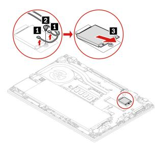
Note: After installation, ensure that you connect the orange cable to the connector labeled Orange on the card, and the blue cable to the connector labeled Blue.
