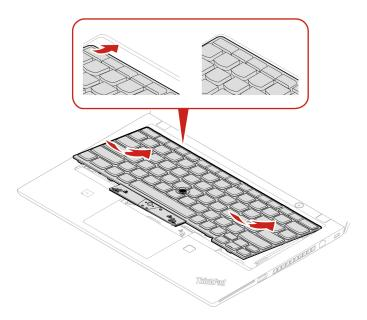
3. Slide the keyboard in the direction as shown by the arrows. Ensure that the latches are secured under the keyboard frame.
