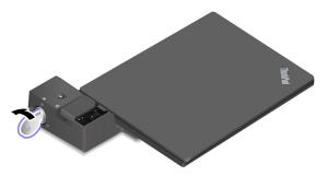
2. Slide the latch in the direction as shown 11 to release the computer, and then grasp both sides of the computer to remove it 2.
