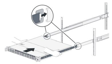
**4** Pull the front latch of the inner rail as illustrated to unlock the inner rail, and continue pushing the chassis towards the rack.
