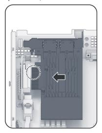
**5** Put the black latch back to the expansion slot to fasten the network interface card.
