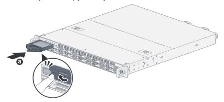
Note: Make sure that the drive tray is completely inserted. Otherwise, the drive might not function properly.
