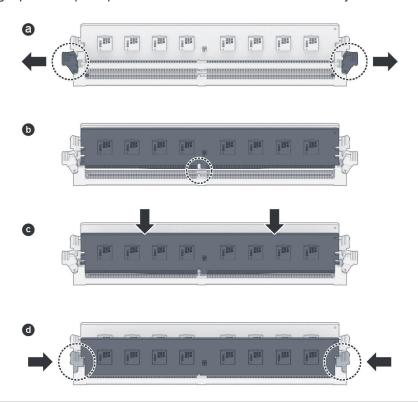
Note: Hold the memory module by its edges and avoid touching the gold connectors.
