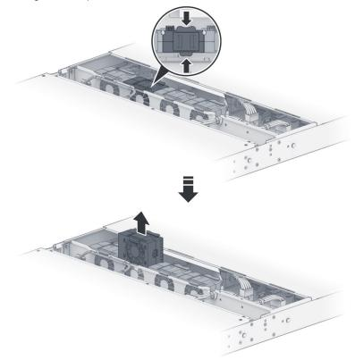
**5** Prepare a new fan and slide it into the your FS2500. Make sure that the fan is aligned properly, as shown below.
