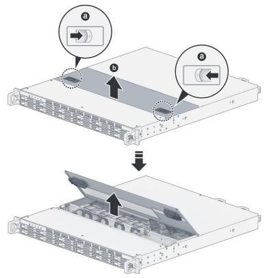
3 Remove the screw on the rear top cover. Slide open the rear top cover, then lift it up and put it aside.
