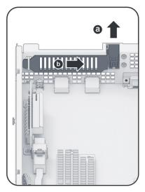
4 Align the card's connector with the expansion slot, and insert the card into the slot.
