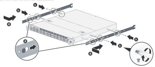
**3** With the help of another person, carefully align the inner rails to the outer rail assembly, and push the chassis towards the rack.
