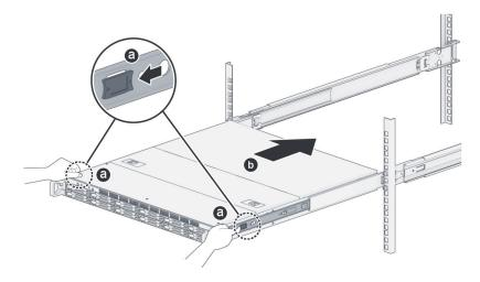
**5** Push the chassis into the end of rack and secure the ear holder to the rack.
