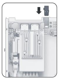
**Note:** Confirm that the connector is fully inserted. Otherwise, the network interface card might not be able to function properly.
