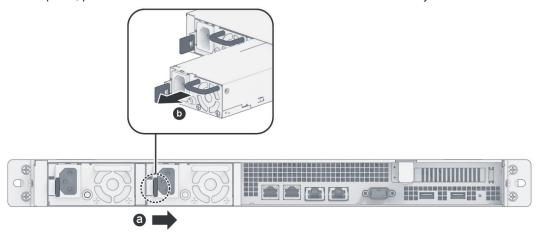
3 Prepare a new PSU. Insert it into the empty slot until you hear a click.
