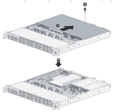
**Note:** When you remove the rear top cover, sensitive internal components are exposed. Avoid touching anything other than the memory assembly when removing or adding memory.
