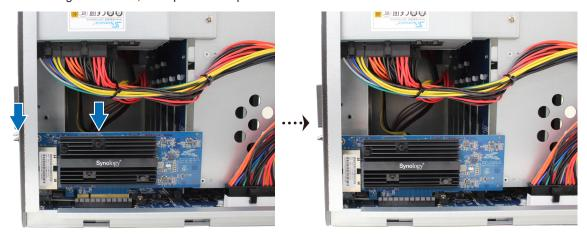
c Push back the clip to secure the newly inserted card.
