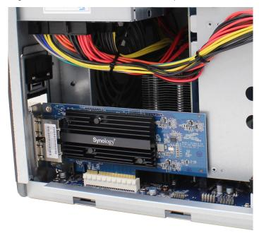
**b** Use two fingers with firm, even pressure to push down on the card and the bracket.
