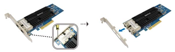
2 Replace the long bracket with a short one, and tighten the 2 screws to secure the short bracket.
