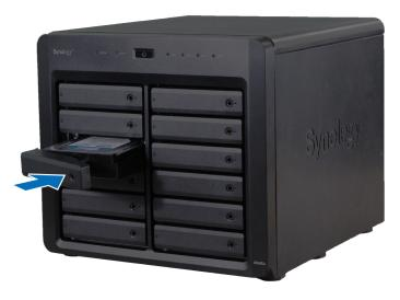
Note: Make sure that the drive tray is completely inserted. Otherwise, the drive might not function properly.
