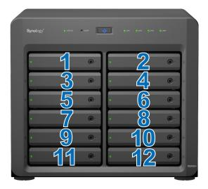
**Note:** If you plan to create a RAID volume, we recommend installing drives of identical size to make the best use of drive capacity.
