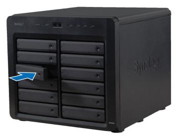
2 Pull out the hard drive tray handle as shown below to remove the hard drive tray.
