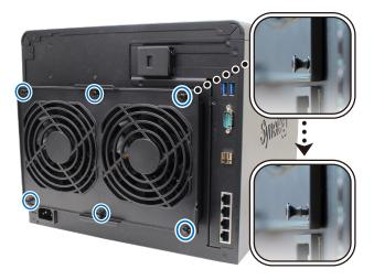
4 Pull out the malfunctioning fan module to remove it from your Synology NAS.
