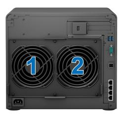
3 Pull the 6 push pins that secure the fan module.
