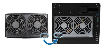
**b** Make sure that all 6 push pins on the new module are pulled outwards before the module is placed into your Synology NAS, and then press the push pins back into place to secure the fan module.
