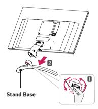
3 As shown in the illustration, pull Screw Cover out to separate it from the set.
