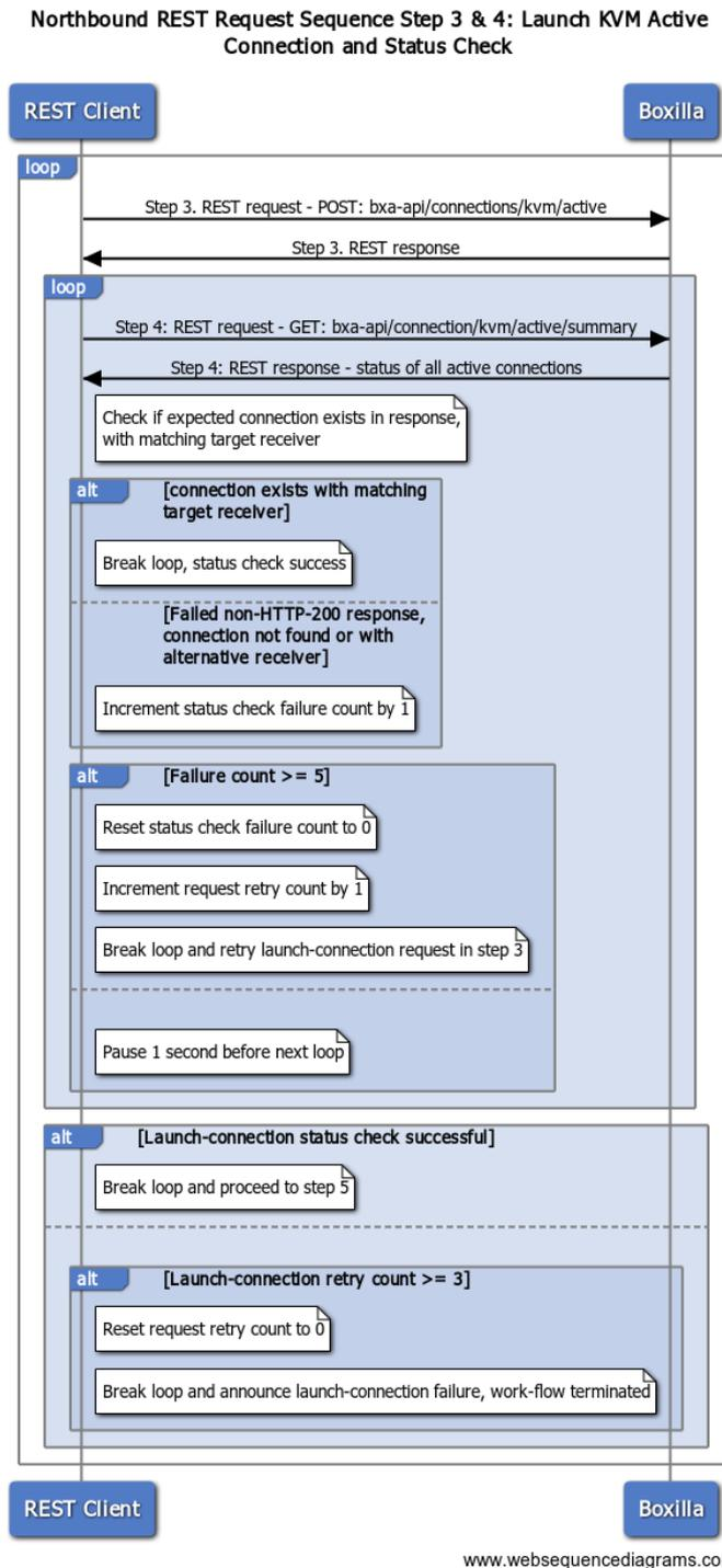
Fig. 2 Sequence of launching KVM active connection and status check (step 3 & 4)
