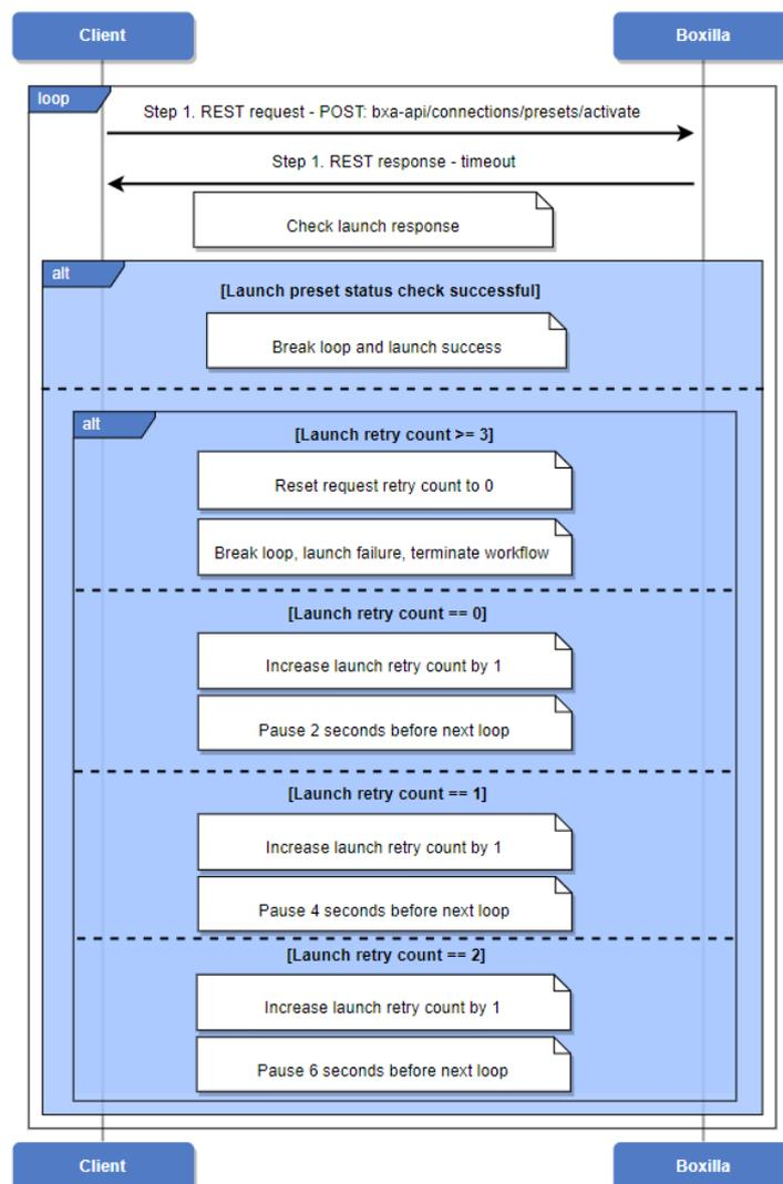
Figure 8 recommended workflow for re-launch preset (timeout)
