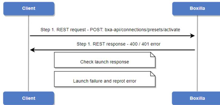
Figure 9 recommended workflow for re-launch preset (400 / 401 error)
