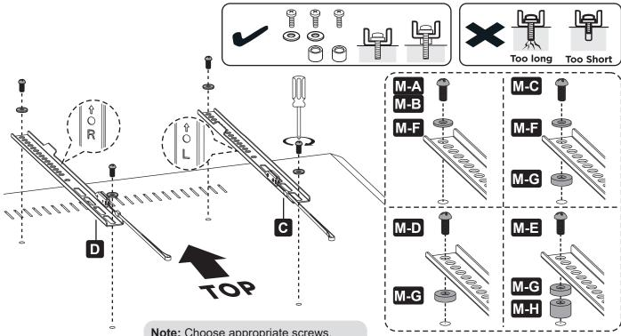
**Note:** Choose appropriate screws, washers and spacers (if necessary) according to the type of screen.
