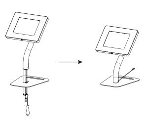
6. Re-configure body segments by removing both middle and lower straight segments. Then re-screw the nuts into the base to remaining curved segment body piece as shown above. Transform your floorstand into a desktop kiosk stand assembly as required.
