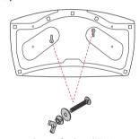
2-Screws for Stand Fixing, 2-Washers for Stand Fixing,
