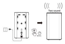
4 Wait until the Wi-Fi light indicator on the top panel turns from a fast blink to a slow pulse. Slow pulsing indicates that the speaker is entering the Wi-Fi setup mode.
