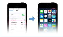
6 After successful Wi-Fi connection, the Wi-Fi light indicator on the top panel will stop pulsing and turn solid. Once you set up this product on your Wi-Fi network, vou can control it from any smartphone or tablet on the same network.
