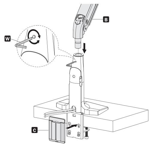
Attaching the Center Mounting Bracket to the Arm
