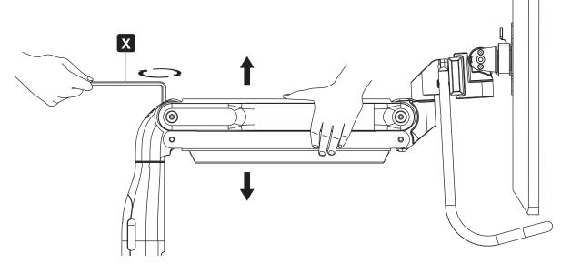
To properly balance the arm with monitors mounted, adjust the spring tension using the supplied hex key as follows:
