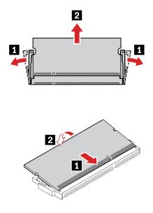
**Note:** During the installation, ensure that you align the memory module to the slot and press down on both ends until the latches are fully engaged with a click.
