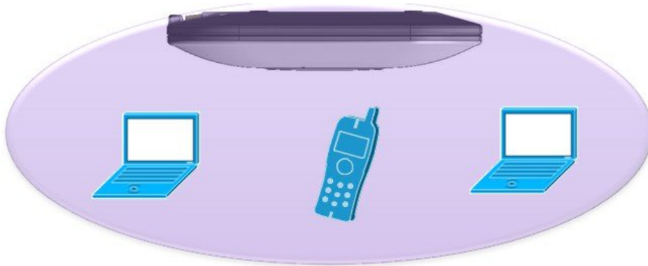
Figure 29: Coverage is optimized for ceiling placement and radiates omni-directionally
