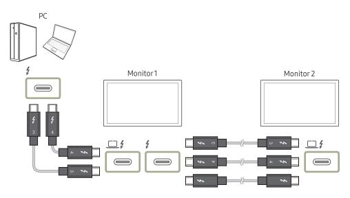
Dual display (daisy chain) support depends on your PC and the connected Thunderbolt<sup>TM</sup> 3 / 4 cable. The Thunderbolt<sup>TM</sup> 3 port on your PC must support dual 4 K @ 60 Hz output, and the particular 40Gbps Thunderbolt<sup>TM</sup> 3 / 4 cable ( $\boxed{\phantom{0}}$   $\boxed{\phantom{0}}$  ) need to be purchased separately. For detailed specification of the Thunderbolt<sup>TM</sup> 3 / 4 cable, visit the official Thunderbolt website.
