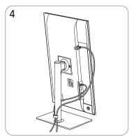
Put both cables in the cable holder on the stand (HOLDER-STAND CABLE) to organize the cables, as shown in the figure.
