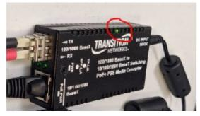
Circled in red above is the location of LED 4 that can be seen inside the metal. LED 4 will turn solid green when the APR function is enabled and is monitoring the fiber link.
