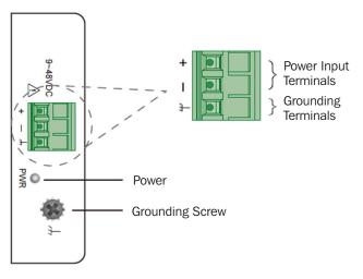
To insert power wire and connect the  $9\sim48$ VDC at a maximum of 0.5A DC power to the power terminal block, follow these steps:
