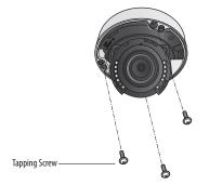
Connect Power and video cables and arrange them through the hole you want to pass when mounting the main body on the mounting bracket, note that not to damage or squeeze the cables.
