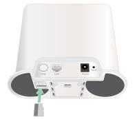
2. Press the edge of the microSD card until it's completely seated in the slot.
