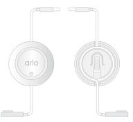
4. Snap the magnetic mount onto the screw and the stopper. The mount clicks into place.
