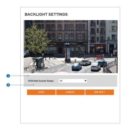
This feature is used when lighting conditions may cause detail loss in the camera's view due to high contrast.
