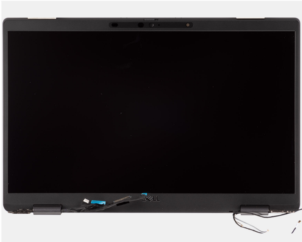
Figure 1. Display assembly with antennae cables
