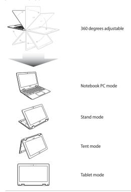
**NOTE:** Rotating the screen to Stand, Tent and Tablet mode will disable the keyboard and touchpad.
