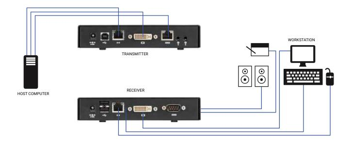
FIGURE 2-2. BASIC EXTENDER APPLICATION
