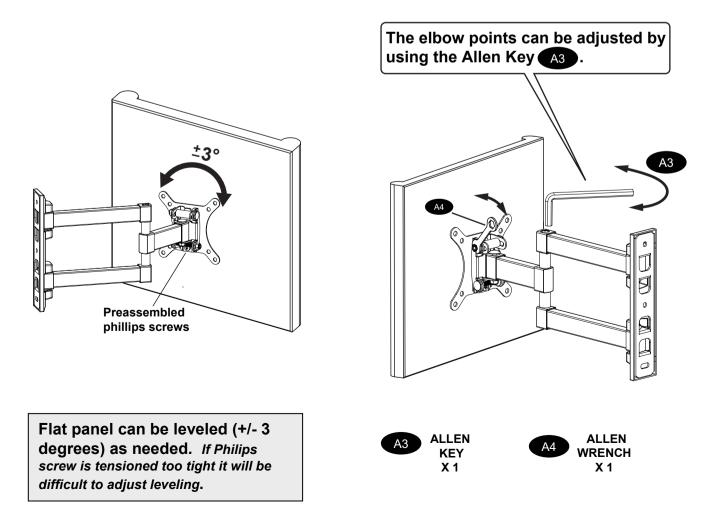
CAUTION: DO NOT EXCEED MAXIMUM WEIGHT CAPACITY. SERIOUS INJURY OR PROPERTY DAMAGE MAY OCCUR! Max Loading Weight: 40 lbs
