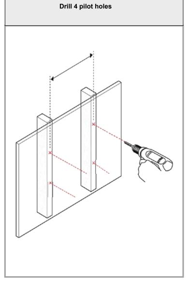
Mount wall plate Coloque la placa de pared Montez la plaque murale
