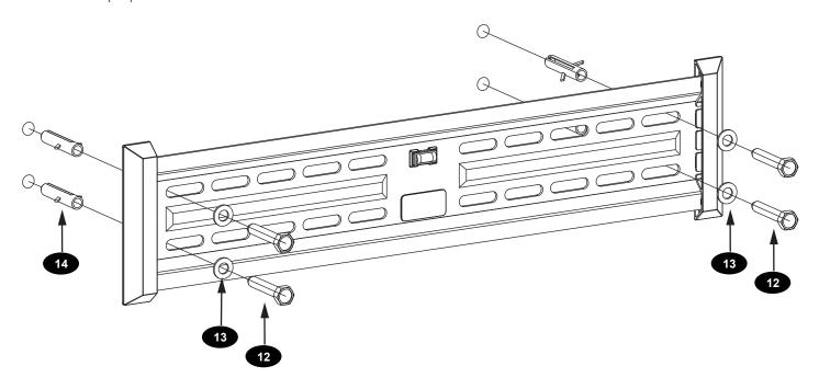
Insert wall anchors gently into concrete wall with hammer if necessary
