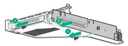
Install the optional riser board in the riser cage.
