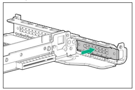
Use a T-10 Torx screwdriver to Install the expansion board.
