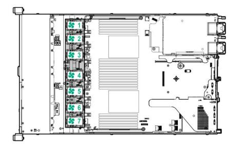
The loss of a single fan rotor (one standard fan) causes loss of redundancy. The loss of two fan rotors (two standard fans or one high-performance fan) causes the server to initiate a shutdown.
