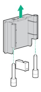
Install high-performance fans in each of the seven fan bays. If needed, ensure each fan is securely installed by pressing the tab. Do not press on other areas of the fan.
