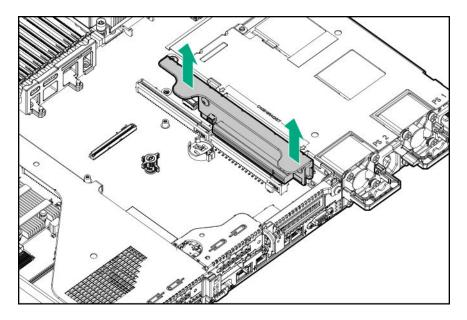
Lift and remove the secondary riser cage latch.
