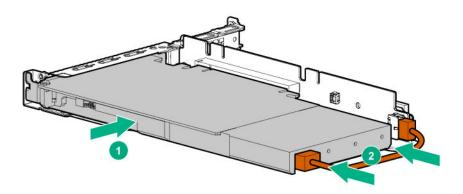
**10.** If the card requires rear support, install the GPU support bracket.
