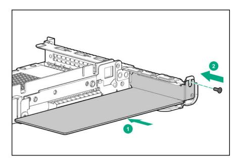
10. Install the primary PCI riser cage (Install the primary PCI riser cage).
