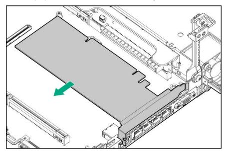
10. Remove the PCI riser cage.
