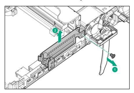
Install the full height PCIe x16 riser cage latch. 9.
