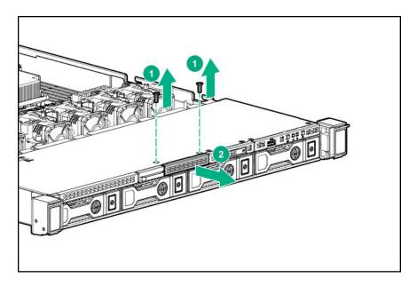
Install the 4 LFF display port/USB module.
