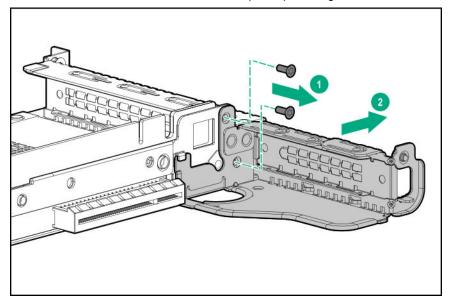
**9.** If needed, install the riser board removed in step 7 on the rear drive riser cage bracket.
