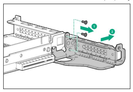
**7.** If installed, remove the low-profile riser cage.
