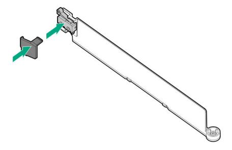
Use a T-15 Torx screwdriver to install the DIMM guard, and then connect the cable to the system board.
