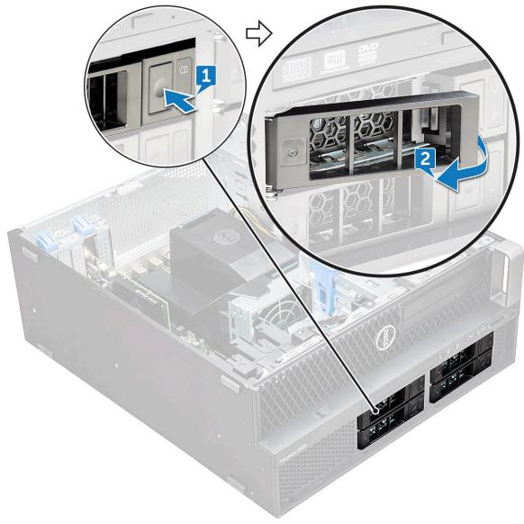
b) Pull the latch to slide the carrier out of the HDD slot.
