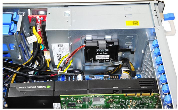
b) Push the securing tab out to release the RAID controller battery.
