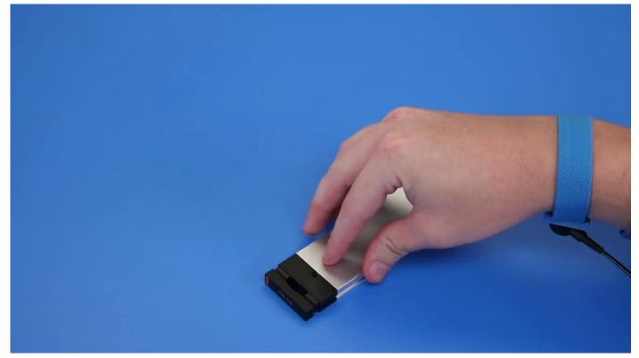
d) Slide the SSD out of the M.2 slot on the carrier.
