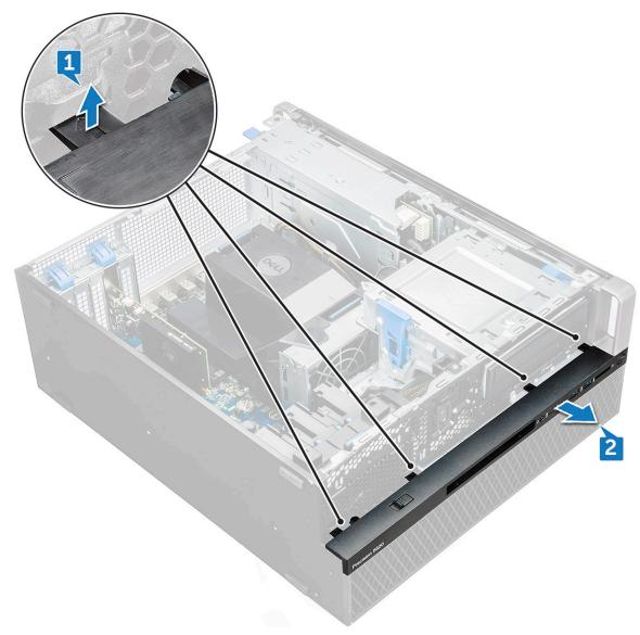
b) Lift the bezel from the chassis.
