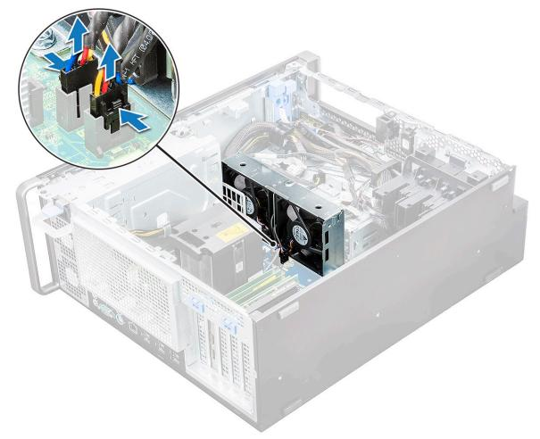
b) Remove the screws [1] securing the system fan to the system board and lift the system fan up [2] .
