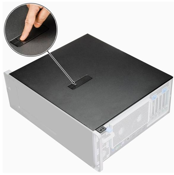
4. Pull the latch [1] upward and rotate it to release the cover [2].
