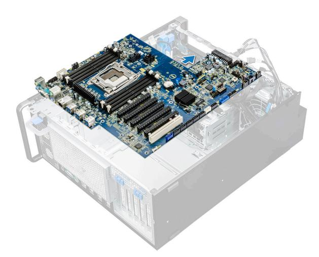
g) Lift the system board up to remove it from the chassis.
