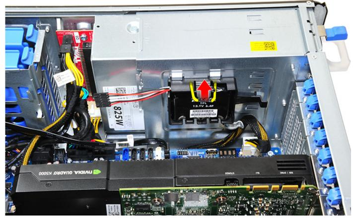
c) Lift and remove the RAID controller battery.
