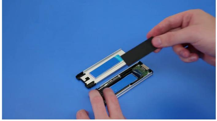
b) Peel off the tape from the SSD carrier.
