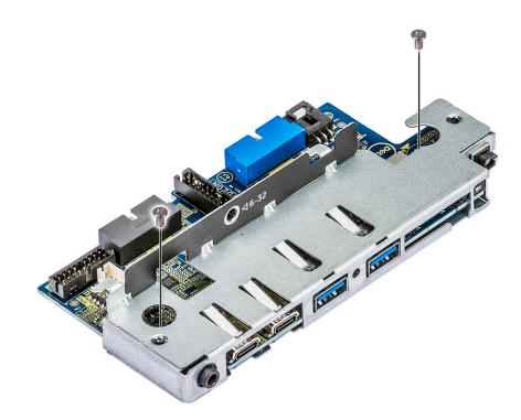
b) Slide the I/O module out of the bracket.
