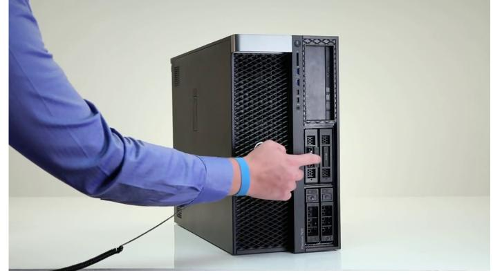
b) Pull the M.2 SSD carrier out of the NVMe flexbay.
