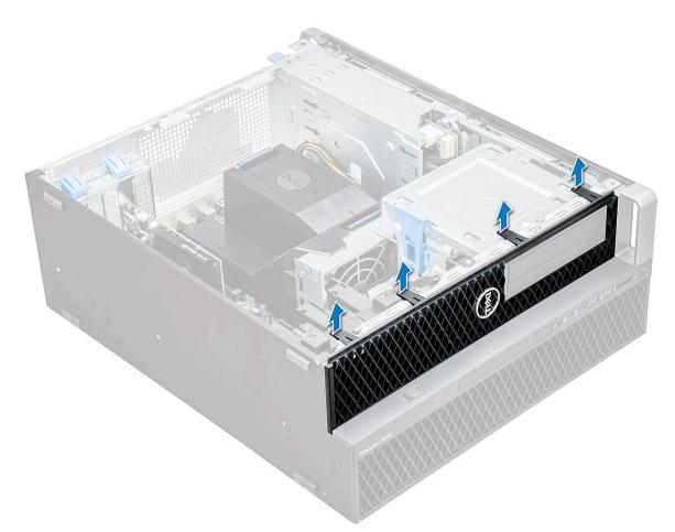
b) Rotate the bezel forward and lift the front bezel away from the system.
