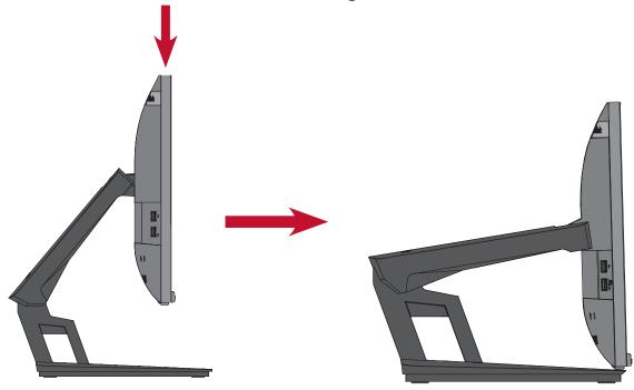
**NOTE:** When adjusting, press down firmly holding the monitor with both hands on the side.
