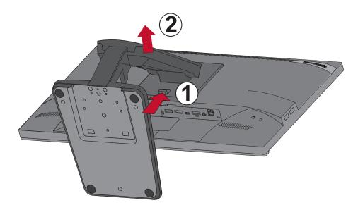
**4.** Pull down slightly to disengage the hooks. Then remove the stand.
