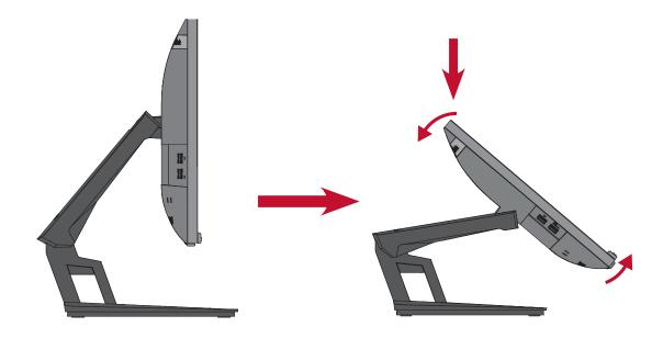
**NOTE:** When adjusting, support the stand firmly with one hand while tilting the monitor forwards or backwards with the other hand.
