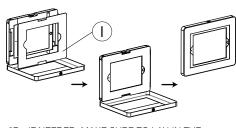
6D - IF NEEDED, MAKE SURE TO LAY-IN THE CORRECT MASKING COVER (I). THEN CLOSE AND LOCK THE ENCLOSURE AND YOU'RE READY TO GO.
