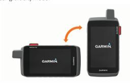
**NOTE:** While using the inReach features of your Montana 700i/750i device, you should use the device in vertical (portrait) mode, with the antenna pointed toward the sky.
