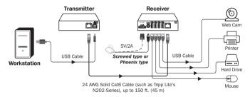
**Note:** When connecting the receiver to power-hungry device(s), add external power (5V 2A) via its Phoenix connector.
