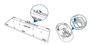
Connect the wireless dongle for keyboard and mouse to a USB port to automatically pair both devices to your ASUS All-in-One PC.
