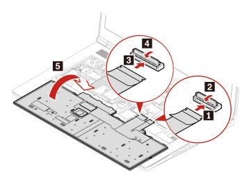
9. Insert the keyboard into the keyboard bezel as shown. Ensure that the top edge of the keyboard (the edge that is close to the display) is under the keyboard bezel.
