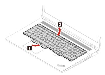
7. Put the keyboard on the palm rest as shown and detach the connectors as **1** to **4** shown. Then, remove the keyboard.
